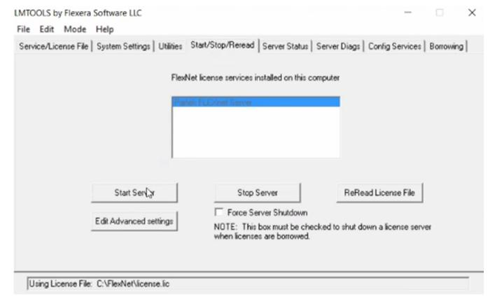
Figure 3. Start FlexNet server
