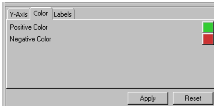
Figure 93: Changing the default colors for Positive/Negative values of the Correlation Profile track
